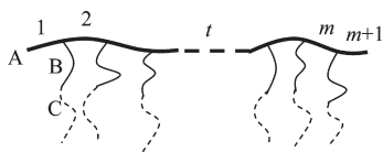
Figure 1. Schematic representation of a comb copolymer molecule. Thick line, thin solid, and thin dash lines represent main chain A and side blocks B and C, respectively.
